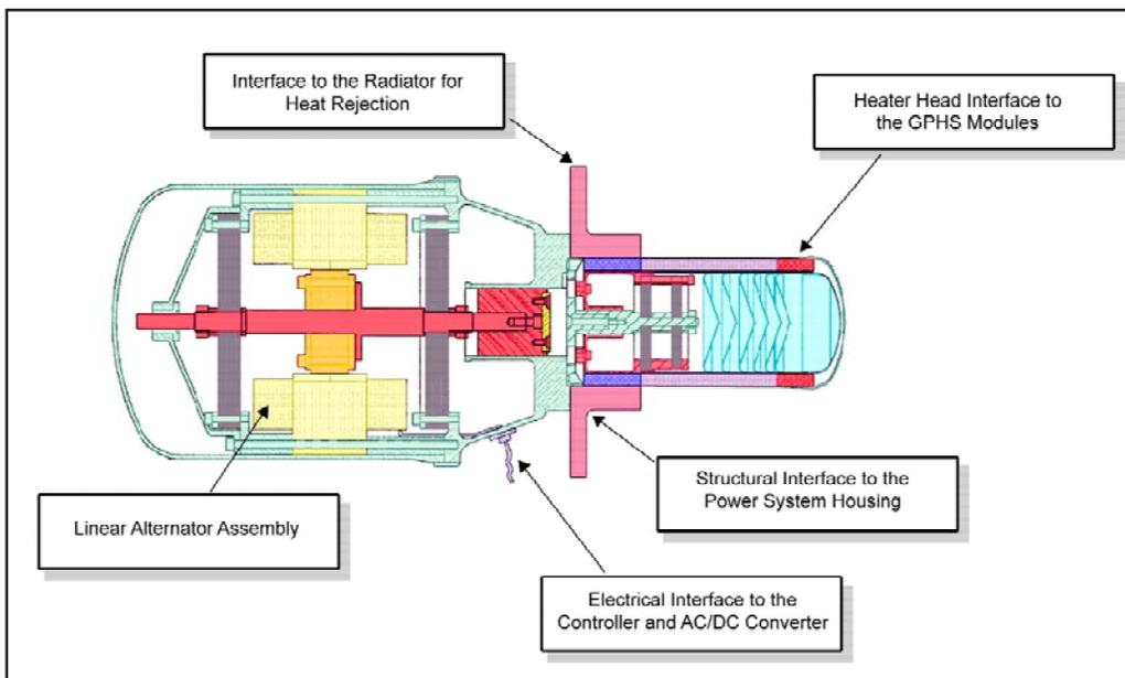
vacuum of space. In addition, it will be designed to deliver 100 to 120 watts of DC electric power. Each SRG will utilize two 55-watt Stirling convertors with about 500 watts of thermal power supplied by using two GPHS modules.
